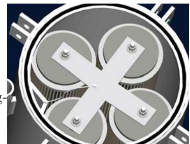
Figure 3. Spider on pre-filter bonded to baffle with braided stainless steel wire.
