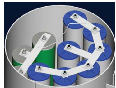
Figure 2. Two spiders in vertical filter/separator bonded together with braided stainless steel wire, bonded to vessel via separator tie-rods.
