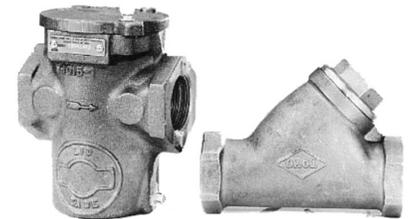
**Y-Strainer** – An inline strainer mounted in the suction line upstream of the pump. The 40 mesh screen strainer protects the pump from damage caused by large particles or objects contaminating the inlet fluid. A screwed port on the strainer allows inspection and cleaning of the strainer element.
