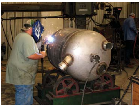
Welding a stainless steel vessel
